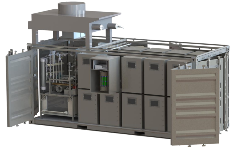
20 ft. container 500 – 2000 kg H 2 /day 450 / 875 bar discharge
